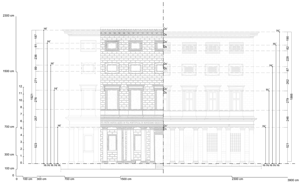
Fig. 6. Comparison process between the Letarouilly survey and the outcomes of the digital metric survey developed in 2018.
