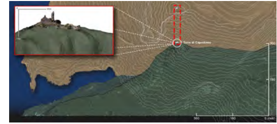
Fig. 2 – Drawing made from processing orthophotos of LIDAR point clouds from the 2009 Extraordinary Remote-Sensing Environmental Plan (Piano Straordinario di Tele rilevamento Ambientale, PST-A), with an integrated nadir view with equidistant lines and orthophoto with vertical frame from the south. In the inset, an image of the mesh model integrated and processed using aerial SfM and LIDAR data.
