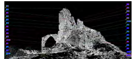
Fig. 8 – Set of TLS point clouds with reflectance values and points used when defining the models.
