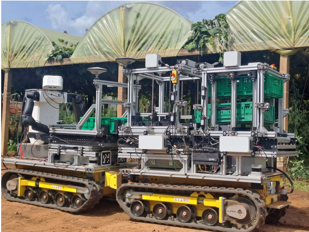
Figure .2. CANOPIES Farming Robot (Left) and Logistic Robot (Right) in Box-Exchange Mechanism Configuration [134]
