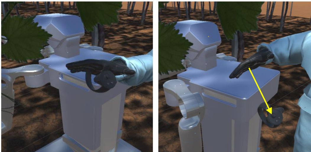
Figure 4.13. Human hand and the controller position without collision vs collision. The yellow arrow indicates the force applied to the robot.
