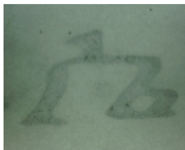
Fig. 09a-b. Codex \Sigma , character se , black ink in LED (a) and NIR (b), images taken with Dinolite Pro2 AD413T-I2V.
