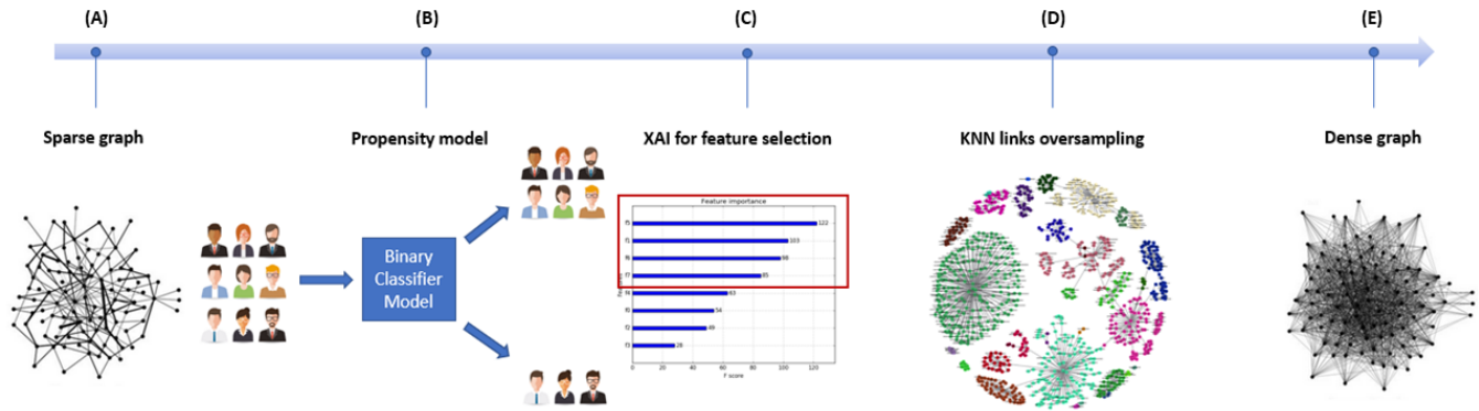
Figure 2: A schematic representation of the proposed framework for graph construction. (A) The initial sparse graph. (B) A propensity model is trained, then (C) Shapley values are computed to select the most representative features. (D) A bipartite graph is built using interaction data, with link augmentation for users and items. Finally, a dense graph (E) is obtained.
