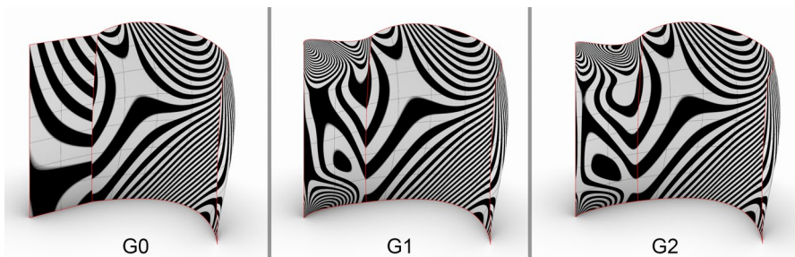
Fig. 5 Study of the reflection behaviour of pairs of surfaces connected in geometric continuity. From left to right: G0, G1, G2
