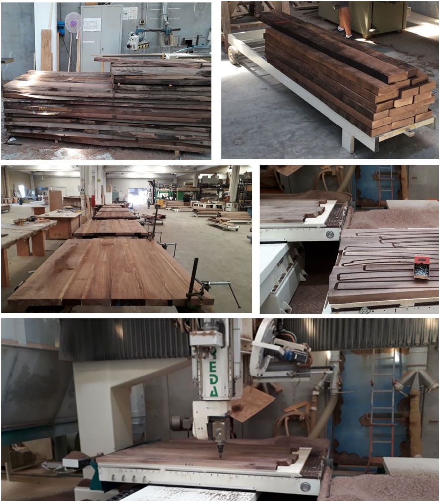
Fig. 10 Construction and assembly stages of the panels used for milling the slats that make up the walls of the installation: from the raw boards to the finished panels used for the processing
