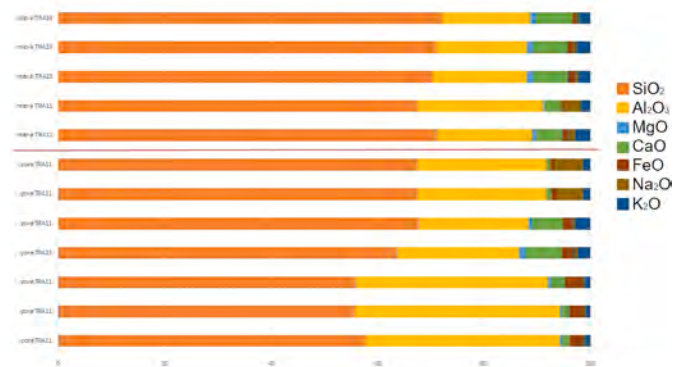
Fig. 7. Bar diagram of EMPA results collected on gel-like matrix (top) and C-A-S-H filled pores (bottom).
