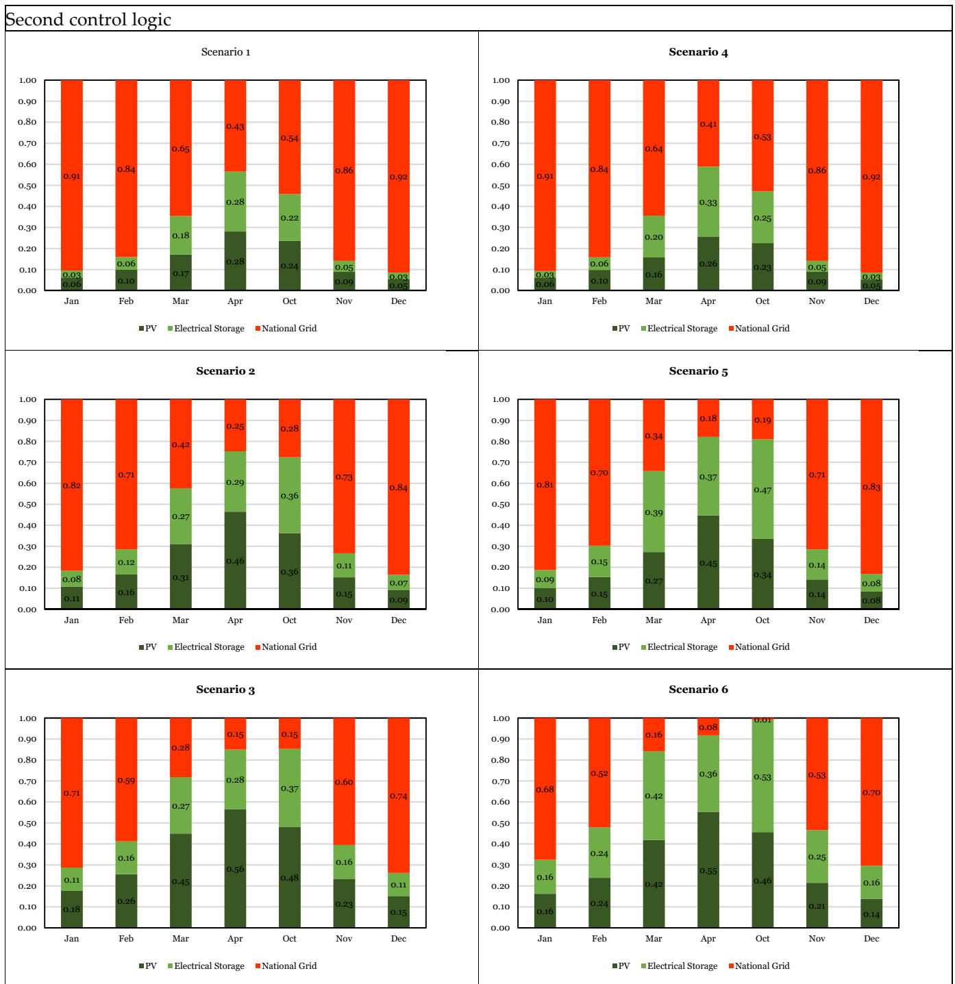
Figure 10. Percentage of load managed by each component varying the scenarios for the second control logic in Milan.
