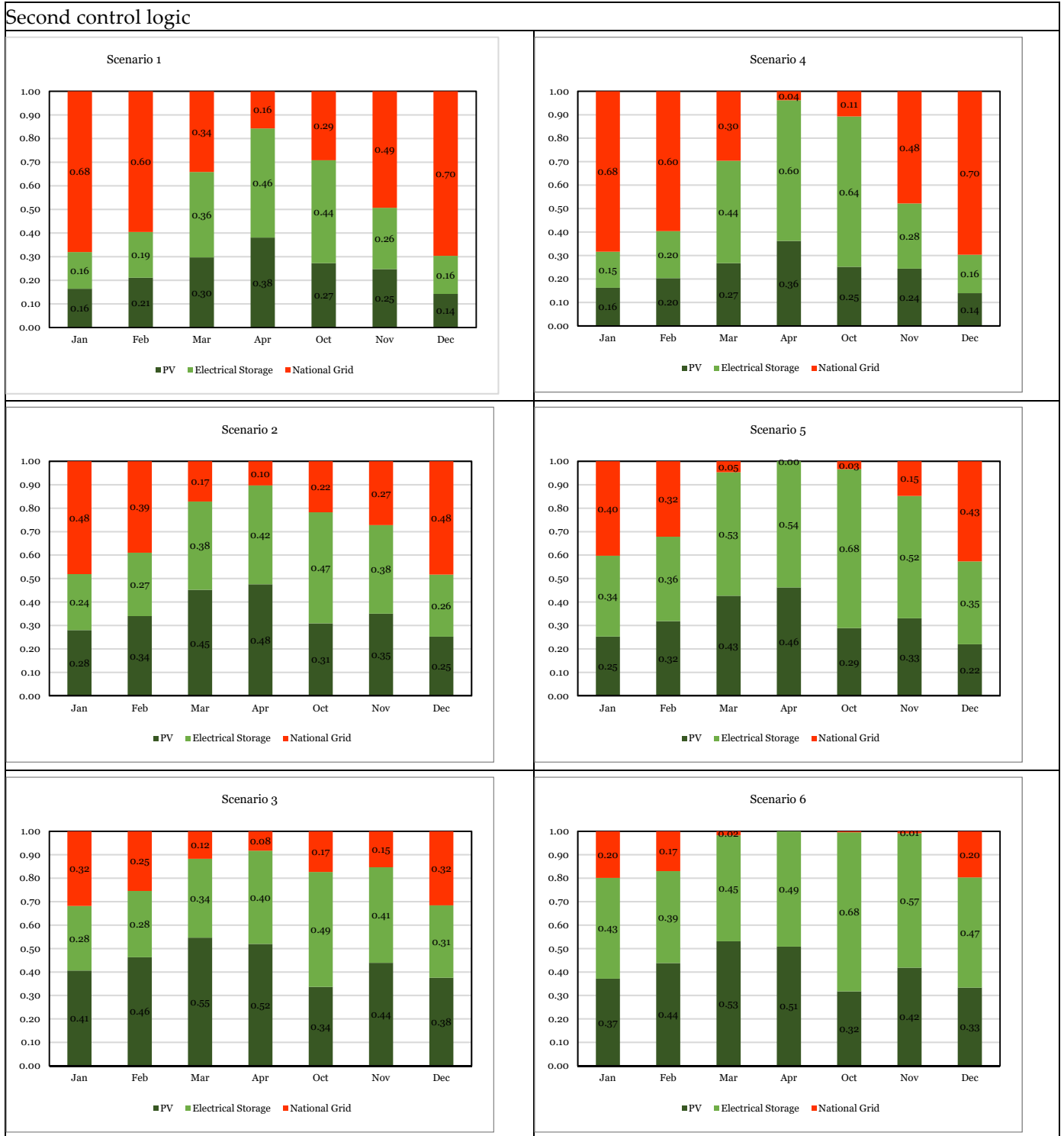
Figure 13. Percentage of load managed by each component varying the scenarios for the second control logic in Messina.
