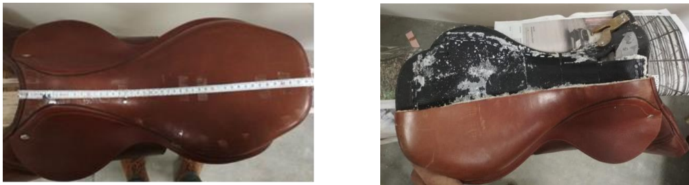
Figure 2: Investigated Horse Saddle: Saddle upper view (on the left); saddletree dissected cross section (on the right).
