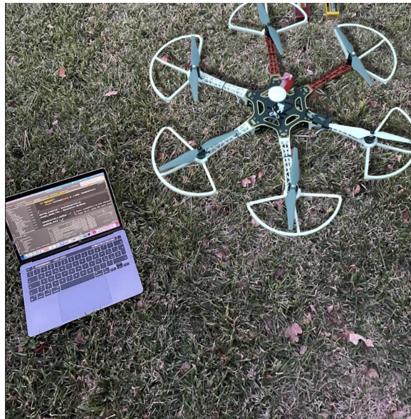
Figure 3.23. BaseStation and DJI F550 Hex-rotor with Naza-M V2
