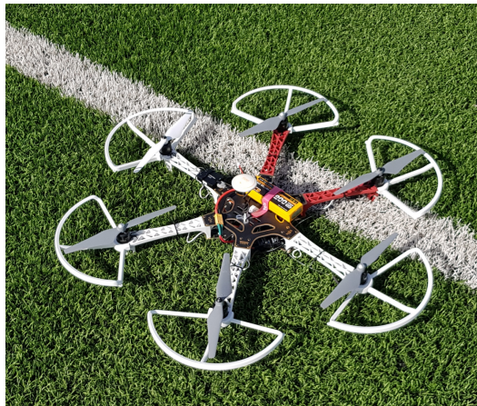
Figure 2.15. DJI F550 Hex-rotor with Naza-M V2
