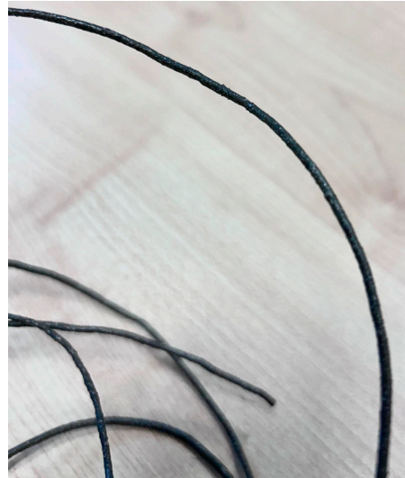
Figure 15. Extruded filament of LDPE-PAL 10 wt%.
