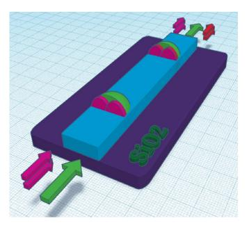
**Figure 21.** Three dimensional illustrative sketch of a high index contrast intermodal waveguide for FWM interaction. The green elements represent the fields on the fundamental modes, while the purple and the red elements represent the fields on the first order modes.
