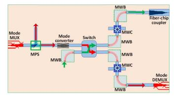
**Figure 18.** A configuration of on-chip MDM links with various multimode photonic devices, including mode (de)multiplexers, mode converters, multimode waveguide bends (MWBs), multimode waveguide crossing (MWCs), multimode power splitters (MPSs), multimode photonic switches, and fiber-chip couplers.
