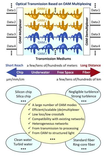
**Figure 5.** Architecture and challenges of the OAM mode division multiplexing communication system towards multi-scale mediums (chip, underwater, free space, fiber).
