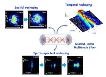
**Figure 13.** Self-shaping of pulses at the output of a nonlinear GRIN MMF; upper left inset: beam cleaning in the transverse x and y dimensions as the input peak power grows from 0.2 kW up to 2 kW. Reprinted figure with permission from [107], Copyright 2018 by the American Physical Society. Bottom inset: beam cleaning in the x transverse dimension and spectral broadening in the wavelength dimension [85]; upper right inset: input power-dependent temporal reshaping at beam center [107].
