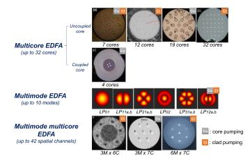
Figure 7. Current state of the art in SDM fiber amplifiers.
