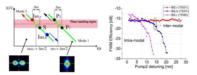
**Figure 22.** Left panel: intermodal four wave mixing scheme using two spatial modes. The green lines represent the inverse group velocity (IGV) curves for each mode. IBS,r and IBS,b are the red and blue scattered idlers, respectively, P1 and P2 represent the pump of the FWM process. Right panel: Bragg scattering FWM efficiency measured for intramodal and intermodal processes. Reproduced from [159]. CC BY 4.0.
