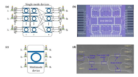
**Figure 19.** (a) The 'demultiplexing-single mode operation-multiplexing' architecture. (b)  $8 \times 8$  multimode switch utilizing demultiplexing-single mode operation-multiplexing. (c) Single multimode device based architecture. (d) Multimode 3 dB power splitter.
