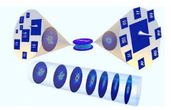
**Figure 12.** Illustrative demonstration of the transformation of the initial (or low power) speckled output beam composed of numerous transverse modes into a nearly bell-shaped beam of fundamental mode sitting of a low intensity multimode background.
