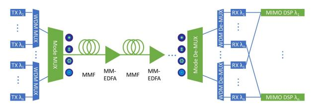
**Figure 1.** Schematic of a wavelength- and space-division multiplexed (WDM and SDM) transmission link using multi-mode fibers (MMFs). Blue building blocks refer to traditional single-mode fiber technology, while green blocks symbolize novel technologies required for SDM transmission in MMFs.
