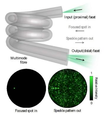
**Figure 14.** *The challenge: overcoming scrambling of optical signals by MMFs.* A focused spot incident on one end of a MMF results in a speckle pattern exiting at the other end that is strongly dependent on fiber configuration. Insets show a simulation of the input focus and the resulting speckle pattern created across the core of the output facet of an ideal MMF, which in this case supports 754 spatial modes.
