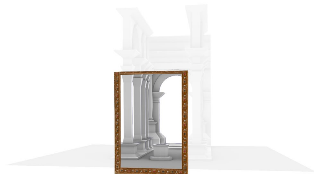
Figure 7. In transparency, the parts of the model do not have to be rendered during the AR experience to achieve the window effect (author's elaboration).
