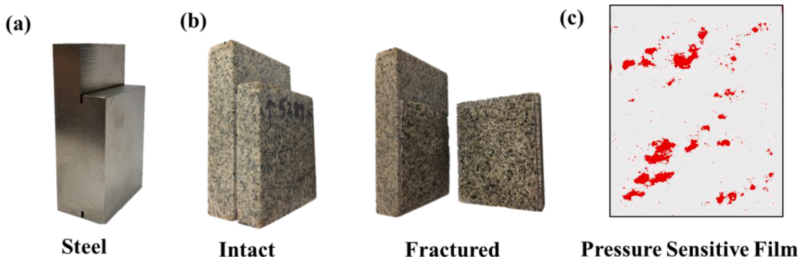
Figure 2. (a) L-shaped steel sample used for calibration; (b) Westerly granite sample first intact then fractured into two halves. The fracture was created using a Brazilian test apparatus; (c) Footprints of the contact areas on a pressure sensitive film showing the distribution of true contacts in red at a normal stress of 15 MPa (experiment p5379).
