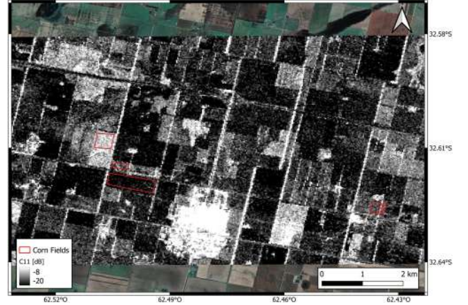
Fig. 3. Monte Buey study site. The C11 element (dB) of the covariance matrix extracted from the first SAOCOM acquisition (13-10-2019) is displayed along with the five corn fields considered for the analysis (red).
