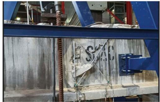
Figure 11. Beam failure-Second Test.
