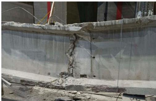
Figure 10. Beam failure-First Test.
