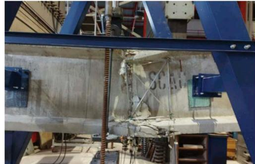
Figure 12. Beam failure-Third Test.
