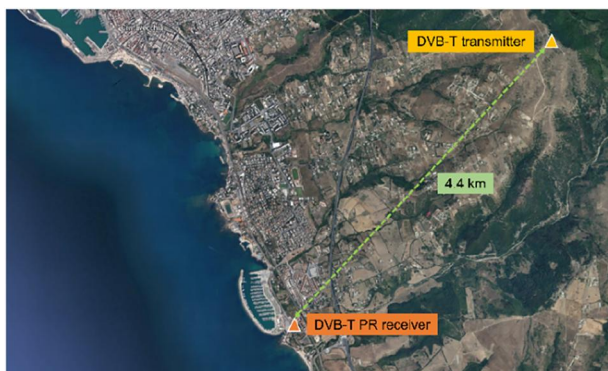
FIGURE 8 Setup for the experimental data acquisition.
