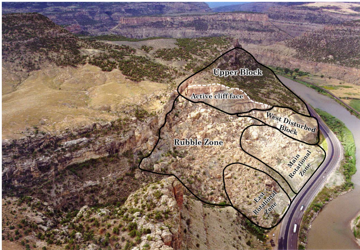
FIGURE 2 Oblique aerial view of the DCL (photo taken pointing to the west direction). The landslide system is divided into different sectors, each one characterized by distinct kinematics (modified after White et al., 2003).
