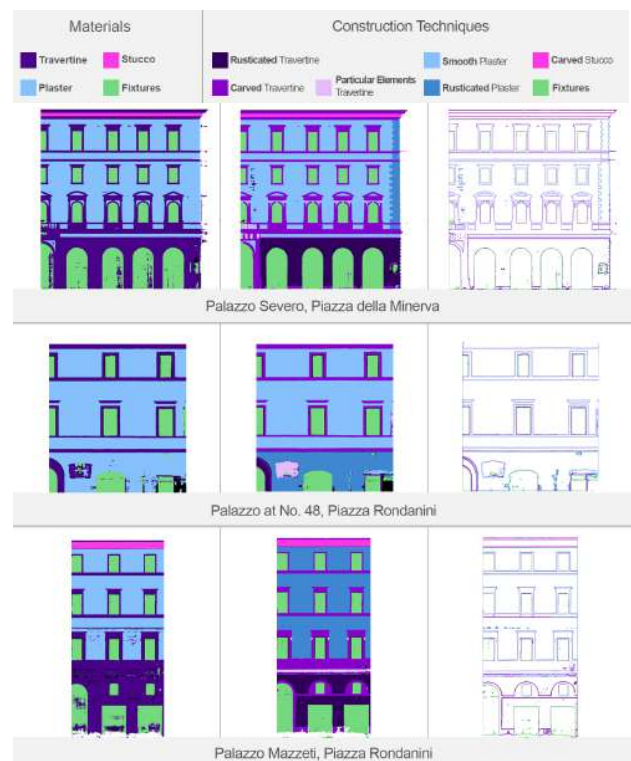
Figure 8: Predicted materials (left) and construction techniques (centre) using the proposed 2D semantic segmentation approach and generated vector drawings (right).
