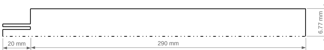
Figure 4.1: Geometry and configuration of the TUMrig 2D in a single-region setting and under the low-Mach number hypothesis.
