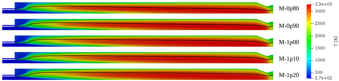
Figure 6.9: Temperature fields for several mass-flows, with superimposed isoline of stoichiometric mixture fraction Z_{st} = 0.2 . Axes not to scale.
