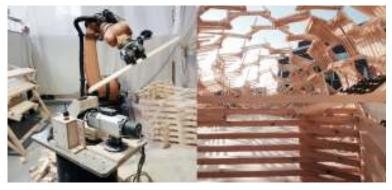
working setup opens up the debate around the fabrication's tolerance: the integration between technical/technological systems and low-engineered setup produces variances between the virtual design and the material actual size pavilion, due to high tolerance.
