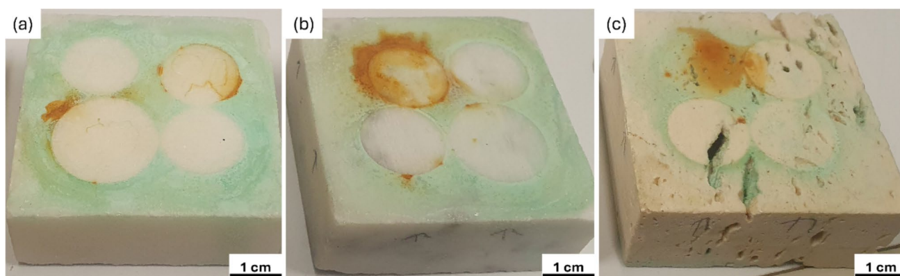
Fig. 2 a Candoglia marble, b Carrara marble and c travertine sample after the artificial staining with metal corrosion products
