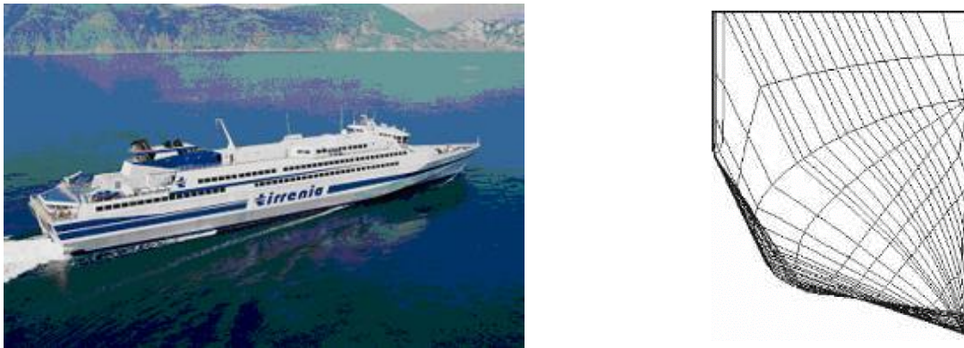
Figure 2. MDV3000 fast monohull: full-scale and bow hull sections.
