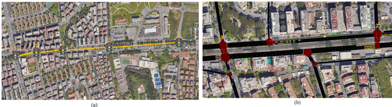
Fig 2. Study area Via Prenestina (a) Sketch of 5 intersections, (b) Microsimulation with dedicated bus lane and pre-signal
