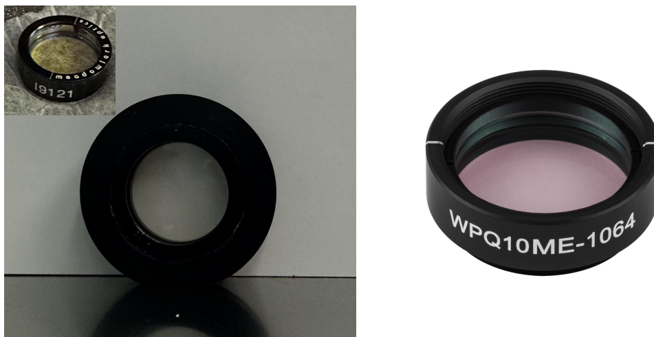
Figure 23 QWP1 , QWP2 : K QWP (left) in its mount for QWP1 and in its plain optic form for QWP2 are Meadowlark I9121 quarter-wave plates. When substituted for MSO-He, the QWPs are replaced with Thorlabs WPQ10ME-633 polymer zero-order quarter-wave plates (right).
