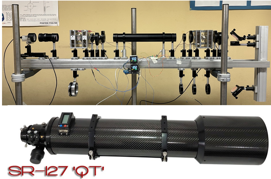
Figure 3.1 Top: TSST-K on the bench at the Solar Station at UTOV prior to its enclosure box mounting. Bottom: TSST-H \alpha telescope.
