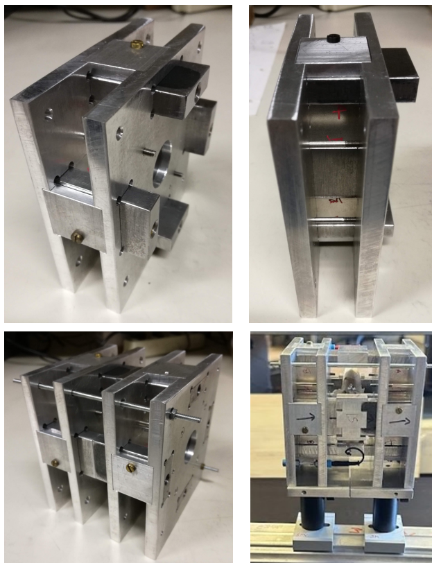
Figure 16 The MOF and WS magnetic enclosures designed to hold the vapor cells at the proper beam height and maintain a constant longitudinal magnetic field via permanent bar magnets. The MOF enclosure has two magnets and the WS enclosure has four magnets.
