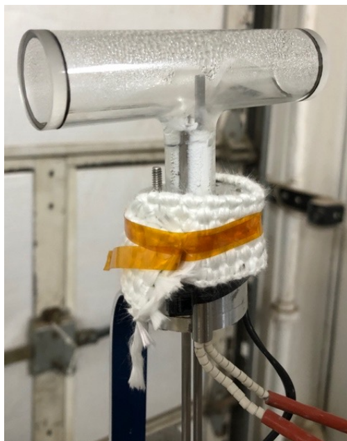
Figure 6.11 Cell connected to vacuum system to grow salt crystals in a clean cell. Saline water was pumped into the cell, and a central drainage tube (metal tube in the center of the cell) was placed for water evaporation. The knit band is connected to a heater to additionally aid in the efficient evaporation of the water. The saline solution was limited to the vertical component of the tube (filling tube) to prevent crystals from forming on the inner cell windows.
