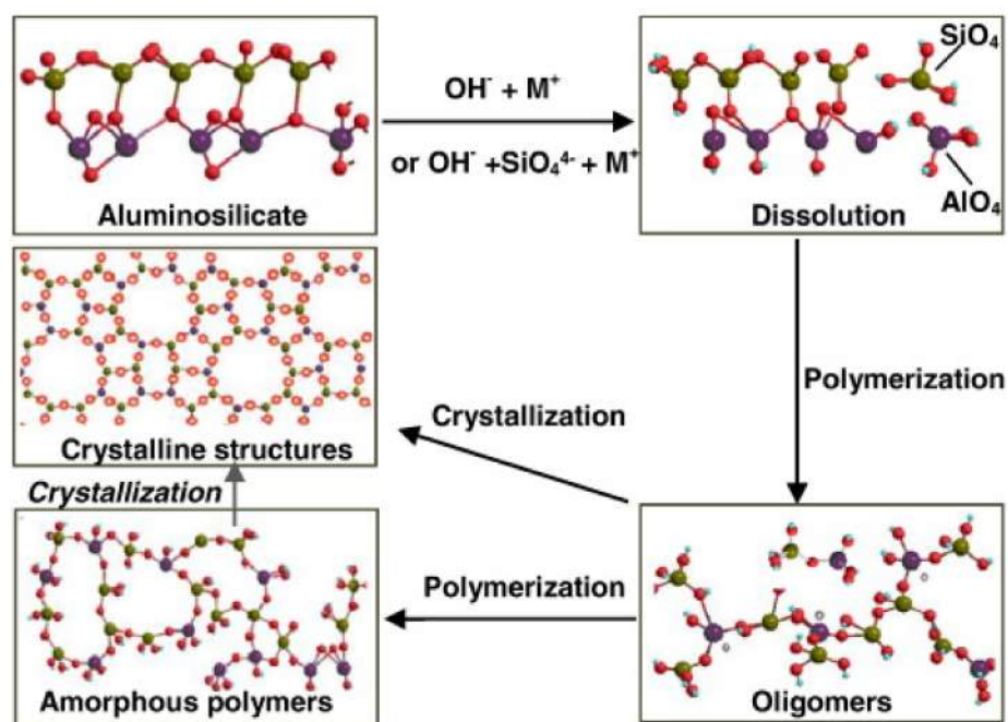
Figure 3. Zhang model of the geopolymerization process. Reprinted with permission from ref. [40]. Copyright 2016 Elsevier.
