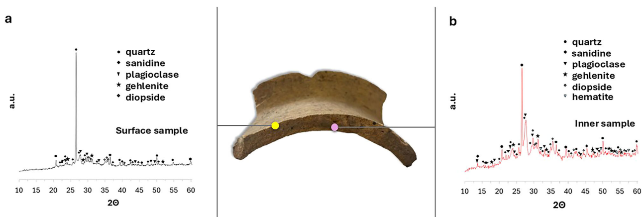
Fig. 6 | X-ray Powder diffraction (XRPD) analysis of the terracotta fragment. XRPD patterns of a the outer surfaces and b of the inner part of the pottery fragment. The main mineralogical phases identified in the diffractograms are indicated.
