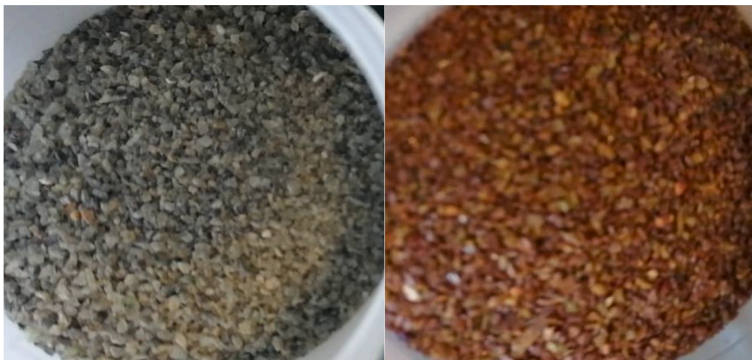
Fig. 3. Illustration of the bed material before (left) and after (right) the gasification.
