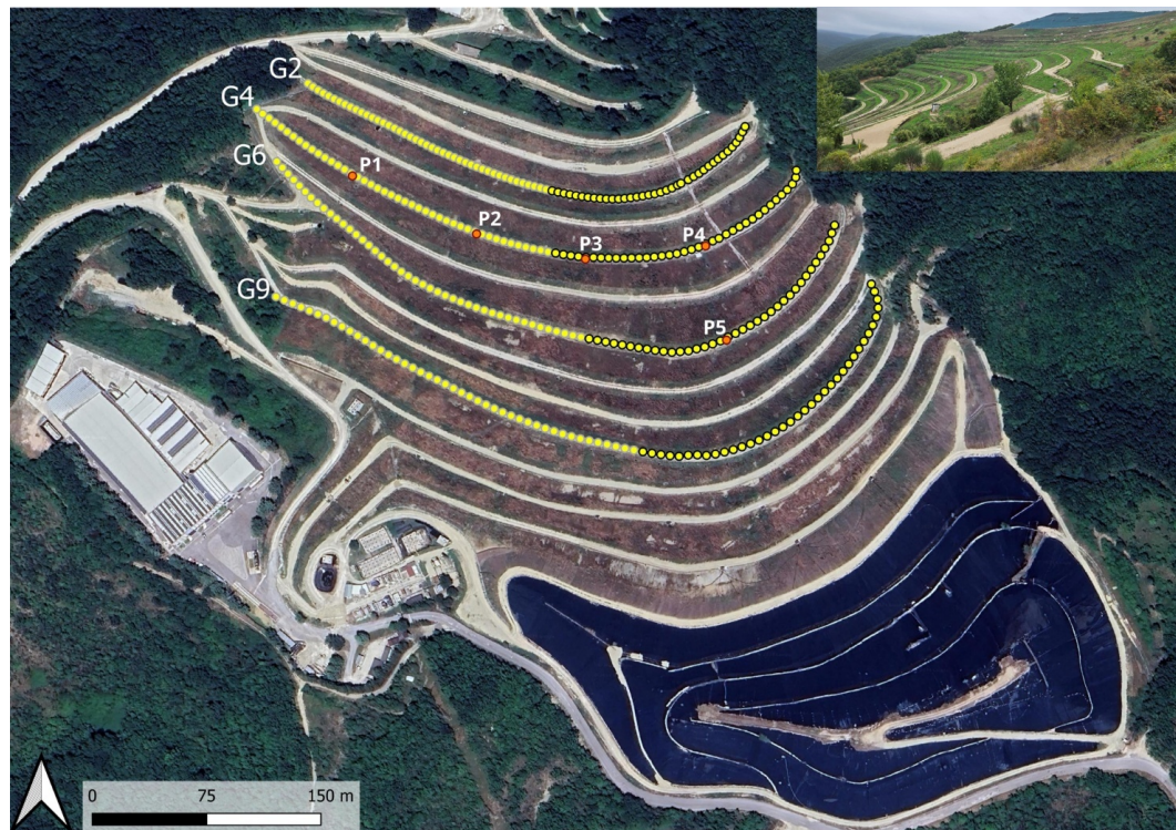
Figure 3.2. Orthophoto of the study area showing the four ERT/TDIP profiles (G2, G4, G6 and G9). Yellow circles mark electrode positions; the subset used for the detailed results is highlighted by a black outline. Orange circles indicate the five piezometers (P1–P5). The inset shows a field photograph of the landfill terraces.
