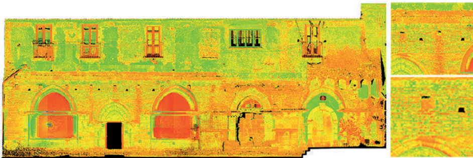
Orthophoto from laser scanning, RGB reflectance 0,18-0,23
