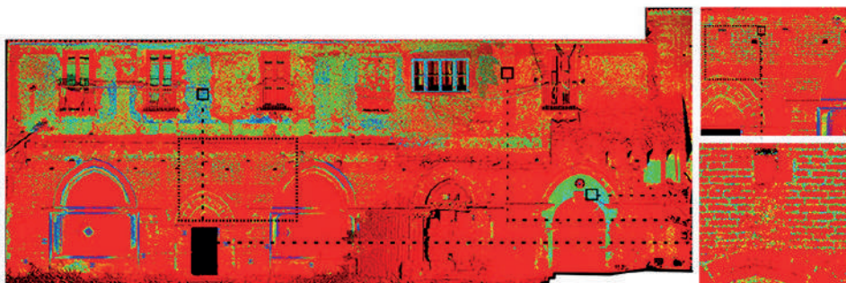
Orthophoto from laser scanning, RGB reflectance 0,35-0,48
