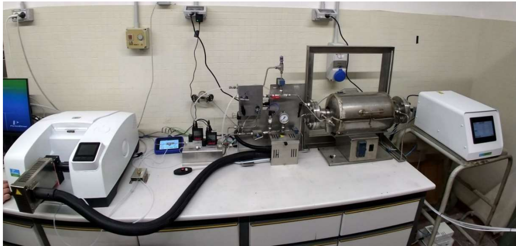
Figure 39: laboratory setup for the thermal abuse test of the Li-ion cell.
