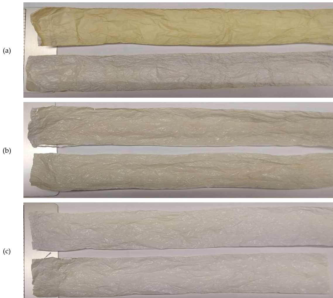
Figure 35: separator foil: (a) C/NCA; (b) LTO/NCA; (c) C/LFP.
