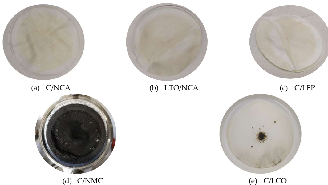
Figure 49: filters collected after the thermal stability test of: (a) C/NCA; (b) LTO/NCA; (c) C/LFP; (d) C/NMC; (e) C/LCO.
