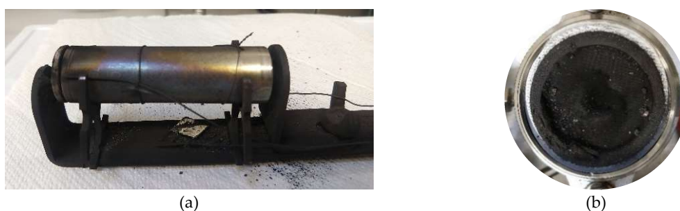
Figure 48: solids collected after the thermal stability test on C/NMC: cell (a); solid ejected from the cell (b).
