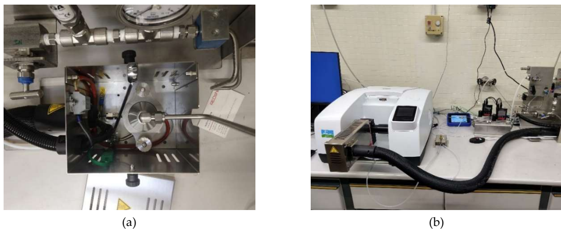
Figure 42: Filter unit (a); transfer line linked to the gas cell of PerkinElmer Spectrum 3 MIR/NIR/FIR.
