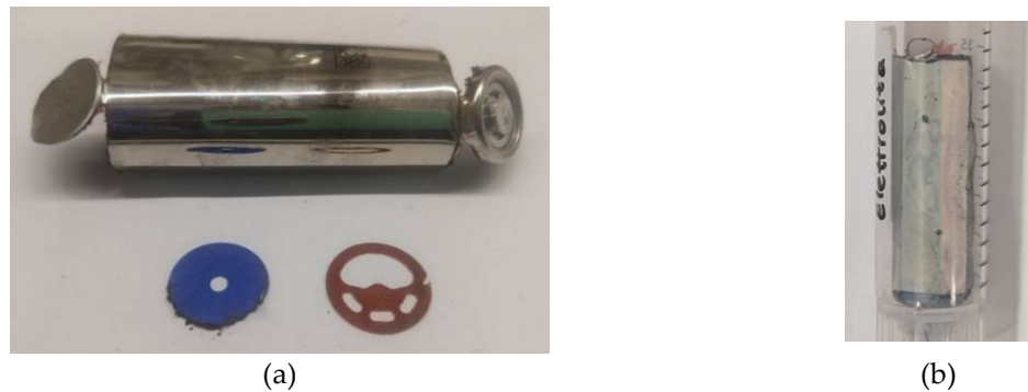
Figure 30: C/NCA components: (a) external case with the safety devices; (b) internal roll.
