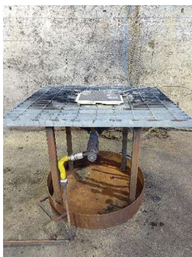
Figure 83: fire test system.
