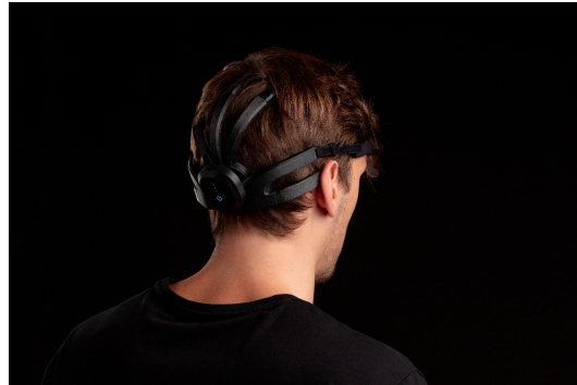
Figure 5. Mindtooth EEG Headset.
