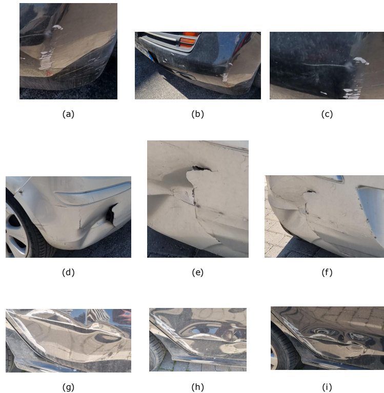
Figure 6.5: Example of damage similarities. Triplets (a)-(b)-(c), (d)-(e)-(f), and (g)-(h)-(i) are real matches of the same damages. Each row shows an example type of damage: scratch , crack , and dent , respectively.
