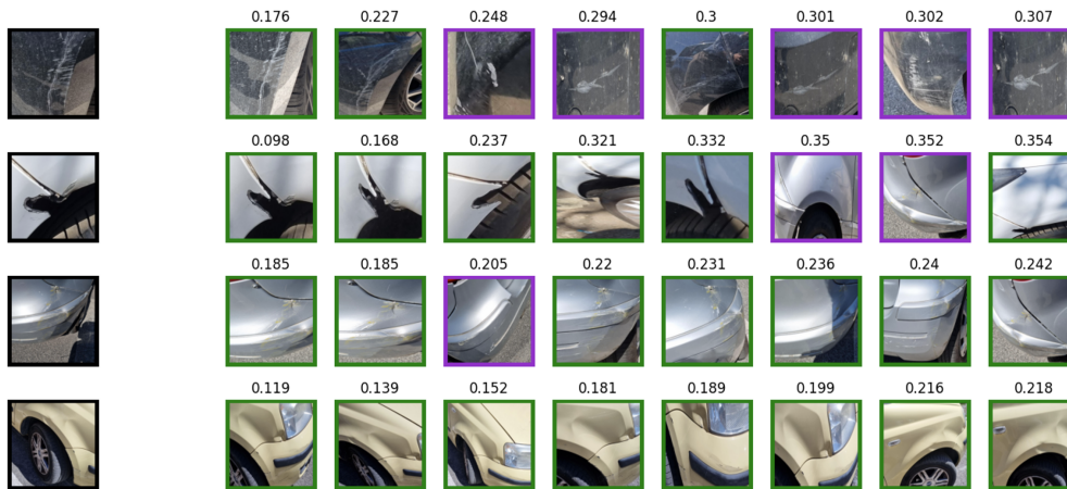
Figure 6.8: Sample queries and matching images in the public test set. The leftmost images are query images, followed by the highest similarity matches. Images framed in green are correct reidentifications, whereas those in purple indicate errors. The similarity score is also shown above each image. Even in cases of error, the model identifies images that are very similar to the query one.
