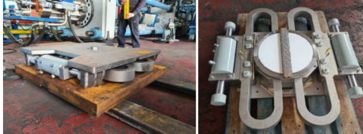
Figure 9. Picente viaduct (Italy). AIOS with shock transmitter. The system consists of a top-placed steel plate connected to the shock transmitter, in turn, connected to the lateral plate of the U-shaped device. In case of slow action (in service), the shock transmitter displacements are allowed, and no force is transmitted to the AIOS. In seismic conditions (dynamic action), the shock transmitter movements are almost restrained, and the AIOS movements are activated.
