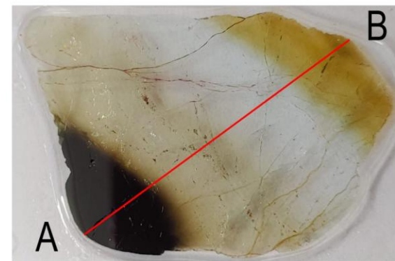
Figure 4.11. EMP analysis of the MAV 4 sample along a straight traverse perpendicular to the c-axis (only selected oxides are reported. See Table 4.4 for complete chemistry.
