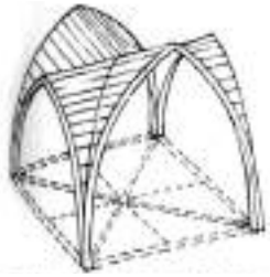
2. Groin vault with straight key lines. The front vaulting has been placed higher.
