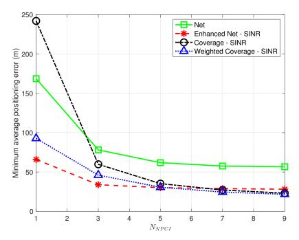
**Figure 12.** Minimum average positioning error as a function of  $N_{NPCI}$  for the proposed strategies using SINR in all strategies but *Net*; the *Single Cell* was not analyzed since, by definition, it operates with  $N_{NPCI} = 1$ .
