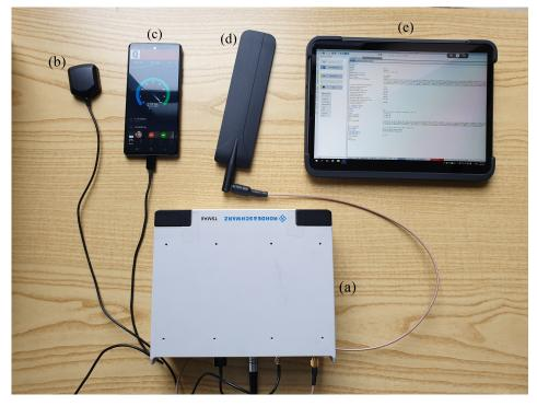
**Figure 1.** The setup adopted for the measurement campaign in Rome, Italy: R&S TSMA6 mobile network scanner (**a**), GPS antenna (**b**), Samsung S20 5G mobile phone (**c**), RF antenna (**d**), and tablet used to remotely access the ROMES software running in the embedded PC within the TSMA6 scanner (**e**) (image drawn from [33]).
