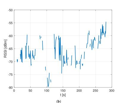
**Figure 5.** RSSI RF data collected for a sample NPCI as a function of time during a measurement run for the Oslo dataset (**a**) vs. the Rome dataset (**b**).
