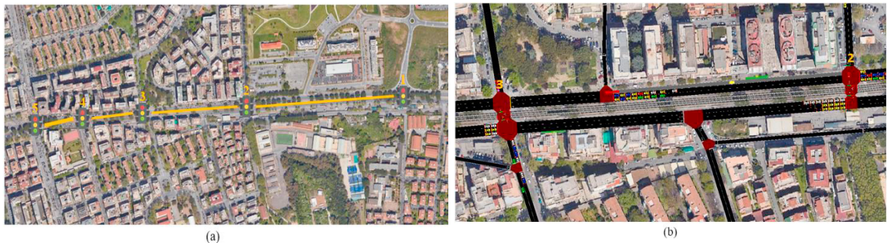
Fig 4. Study area Via Prenestina: (a) Sketch of 5 intersections, (b) Microsimulation with dedicated bus lane and pre-signal.
