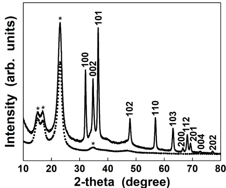
**Figure 2.** XRD patterns of flax (dotted curve) and ZnO-coated flax fibers (solid curve) as fabrics. \* Peaks attributed only to flax fibers.
