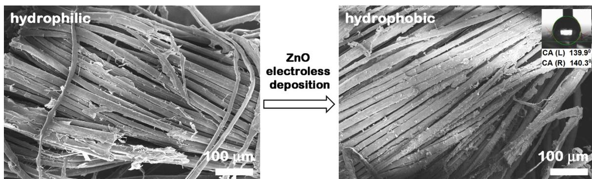
**Figure 5.** FESEM images of flax and ZnO-coated flax fibers as fabrics. In the inset is shown the optical photograph of the water droplet shape on the hydrophobic surface of ZnO-coated flax fabrics and the water contact angles for the corresponding sample.
