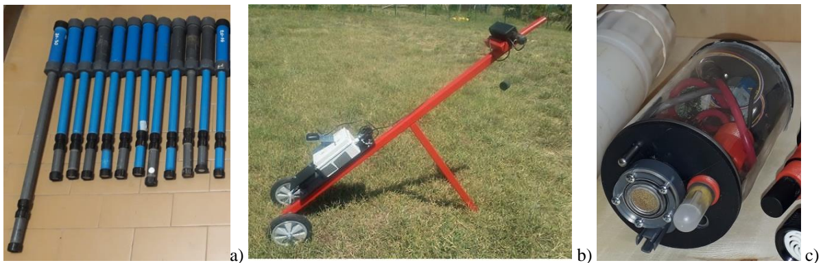
Fig. 1. Photographs showing: (a) various GasPro sensors ready for deployment at different depths in the unsaturated soil horizon (note that the sensor is located in the bottom end while batteries, control electronics and Wi-Fi antenna are housed in the wider, upper tube); (b) the Ground CO 2 Mapper; and (c) the Multipla groundwater monitoring probe.
