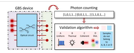
**Figure 1.** GBS validation. In the GBS paradigm *n*-photon configurations are sampled at the outputs of an optical circuit with *m* ports. The aim of a validation algorithm is to exclude that the obtained samples could have been generated by classically-simulable models. Previous experiments mainly focused in techniques capable to rule out the uniform sampler, the thermal, coherent and distinguishable SMSV states hypotheses.
