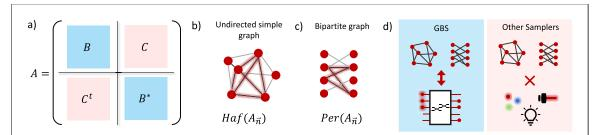
**Figure 2.** GBS and graph perfect matching. (a) Structure of the  $2m \times 2m$  sampling matrix for m independent Gaussian states injected in a m-port interferometer. (b) The hafnian as the operation to count the perfect matchings, highlighted in red, in a simple undirected sub-graph  $A_{\vec{n}}$  with n=4 nodes. (c) The permanent as the same operation for a bipartite graph. (d) The adjacency matrix of undirected graphs, even in the bipartite case, can be encoded in GBS devices.
