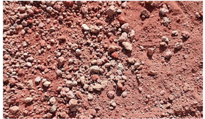
Fig. 2. “Red Pozzolana” used as basic constituent of the mix ground for martian soil reproduction.
