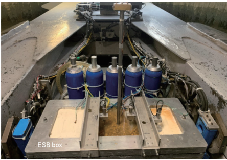
Fig. 2. Reduced-scale model loaded on the centrifuge.
