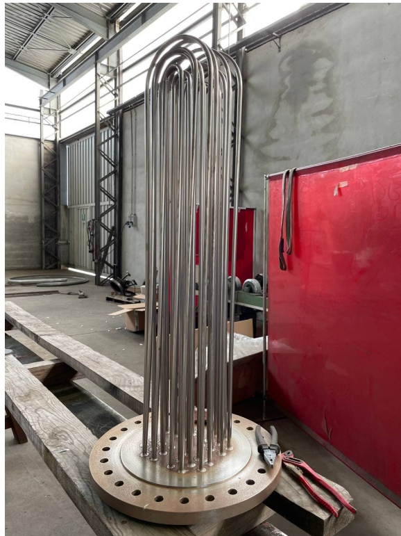
(a) Picture of the niobium tube bundle
