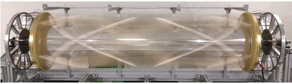
Figure 1: The MEG II drift chamber. The drift chamber is still mounted on the assembly structure in the clean room, the two carbon fiber support half-shells are not yet mounted
