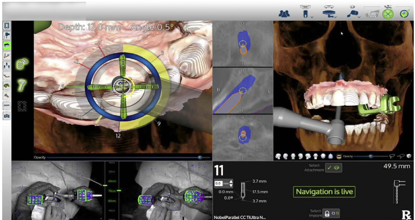
FIGURE 4 Navigation system screen during the dynamically guided implant drilling and positioning. The blue track indicated the implant trajectory planned in the software. The window on the right showed the 3D interplay between the surgical handpiece and the rendering of the patient anatomy. The window on the left showed the 360° control on the implant trajectory and depth
