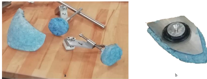
Fig. 6. a) Resin bronze-frame interfaces; b) particular of the back of the left leg interface.
