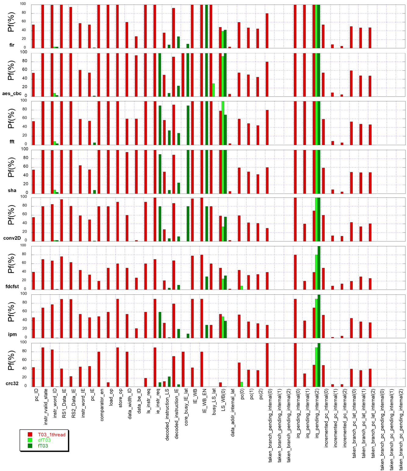
FIGURE 7. Fault injection results with a time frame spanning approach for the T03, fT03, and dFT03 cores. Target registers on the horizontal axis and failure probability (%) on the vertical axis.
