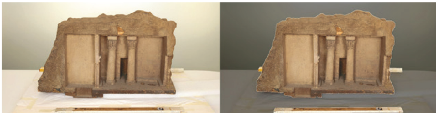
Fig. 5 - Masking of the images: (left) image as acquired, (right) image with mask on the background
