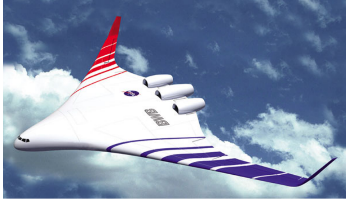
Figure 2: The new concept of aircraft by NASA: The Blended Wing Body, Ref. [2]
